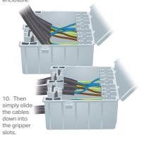
11. Repeat installation process for left hand side of the WAGOBOX XL. The example below illustrates how the WAGOBOX XL can be used to connect a switching circuit (right side) to four light fittings (left side).
