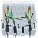
6. When a large number of cables need to be connected on a single circuit then the central receptacle can be used to connect the cable earth wires together using the 2273-208 PUSH-WIRE® connectors and jumper bar 862-482.
